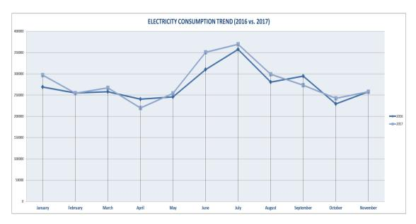
As shown in the chart above, the energy consumption trend in 2017 is almost overlapping with 2016, although the 2017 line jumps up in correspondence with the summer months (May, June, July and August), which traditionally register the most intensive consumption of electricity due to the switch on of air conditioning systems within the EUI Campus (24 May for 2017). A detailed monthly analysis shows a substantial increase, corresponding to +3,29% for the month of May
